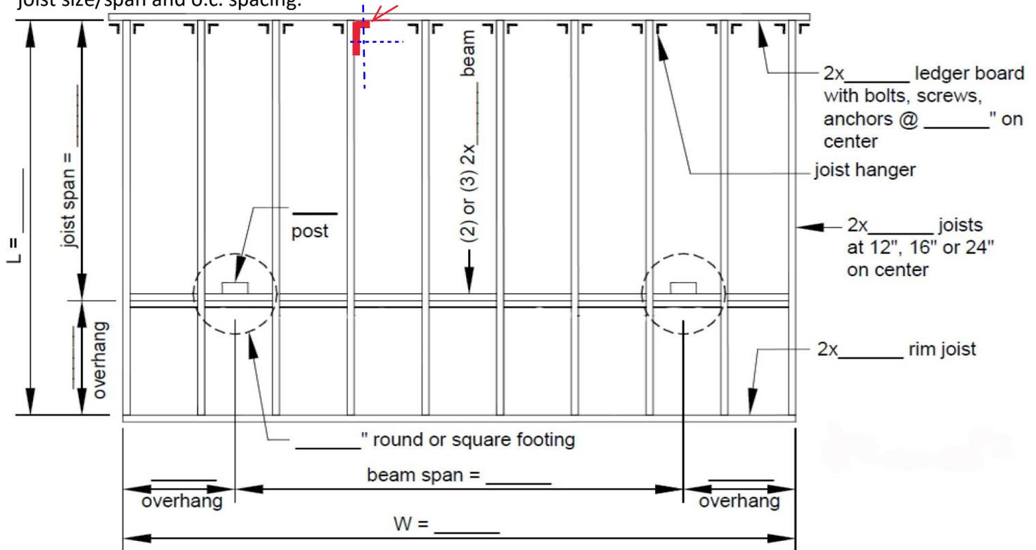
**DECK CROSS SECTION:** Submit one (1) copy of a deck construction cross section. Make note of ledger type, existing house wall materials/connection details, post to beam connection details, post/beam/joist sizes.
